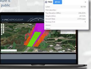
Built-in tree growth rate tool and survey data quickly identifies key attributes of any obstruction.
