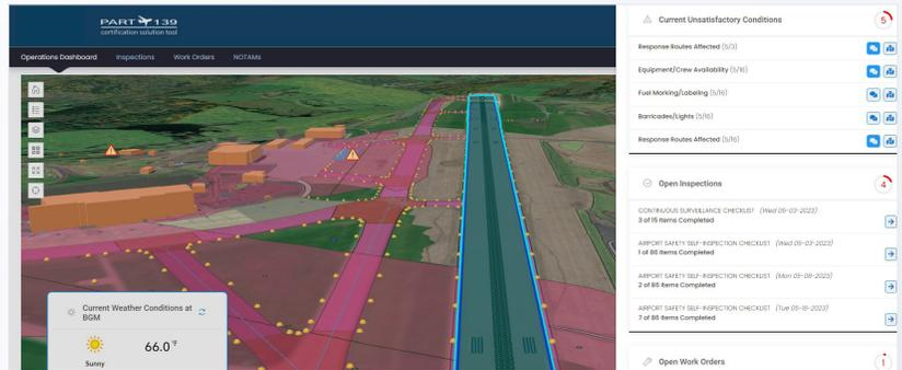
The Operational Dashboard provides a snapshot of airfield assets and maintains data for monitoring and reporting
